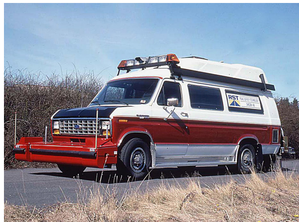
Figure 12: The highspeed Road Surface Tester
