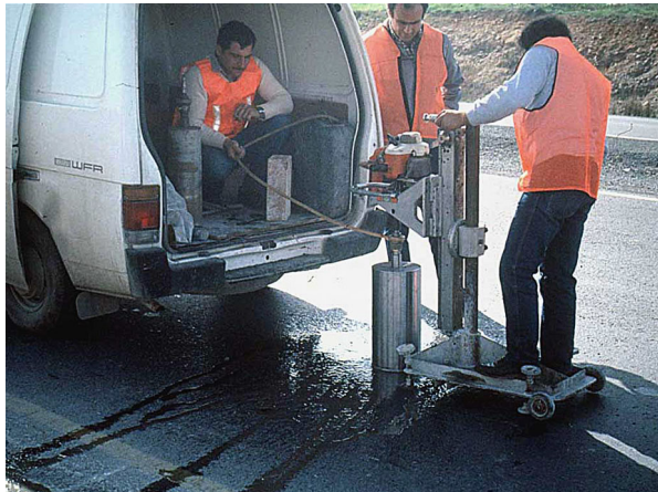
Figure 14: Cutting cores for detailed investigation
