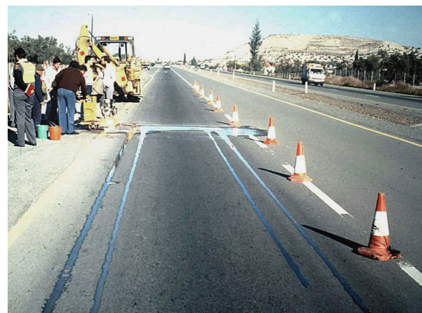
Figure 8: Ruts in the wheel paths
