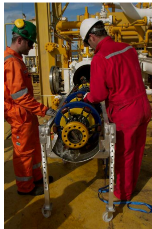
Figure 6: Example of pig for specialist application [from http://www.pipeline-pigging.com with permission from S Hutcheson, Pipeline Pigging Technology Limited].
