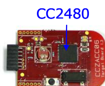
Figure 3: Z-Accel demonstration board with the CC2480 ZigBee 2.4 GHz network processor [from www.ti.com ]
