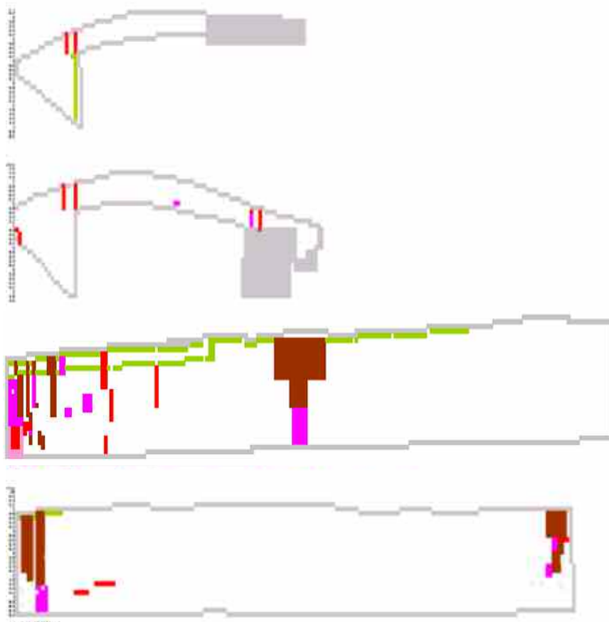
Figure 14: Results of onsite inspection translated into a defect map (top to bottom – north external wall, south external wall, west internal wall, east internal wall). For key see text.
