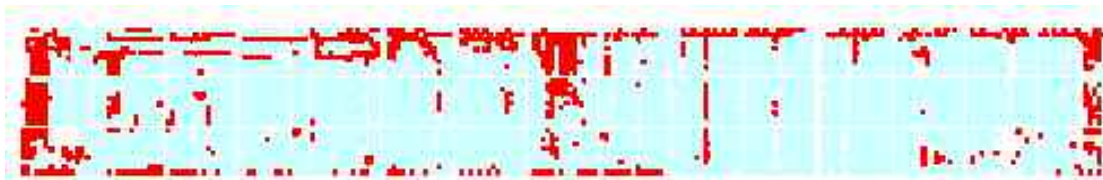
Figure 30: Combination of discriminant function results and initial segmentation. (individual images, Winnersh bridge, west face). Blue = zero reported by both initial segmentation methods; Red = classed as a defect / feature by discriminant, and not ruled out by initial segmentation.
