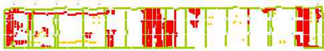
Figure 31: Manual image analysis reference data (individual images, Winnersh bridge, west face). Red = 'Defects'; Green = 'Features'; Yellow = 'Other'
