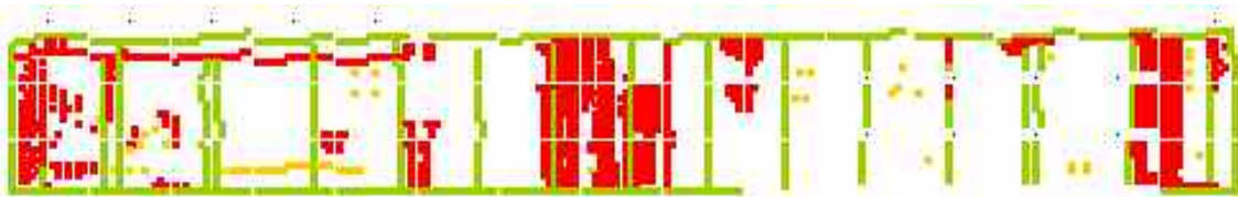
Figure 26: Manual image analysis reference data (individual images, Winnersh bridge, west face). Red = ‘Defects’; Green = ‘Features’; Yellow = ‘Other’
