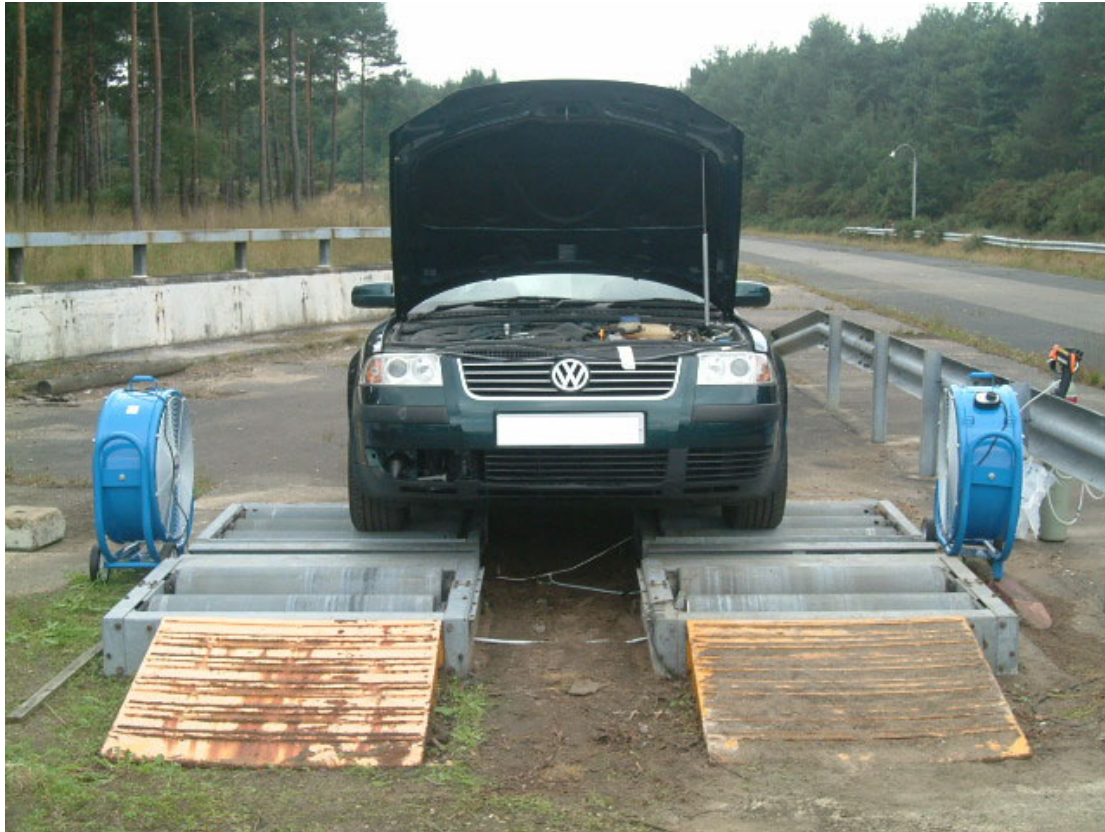
Figure 2: Frontal image of Passat car mounted on the rollers
