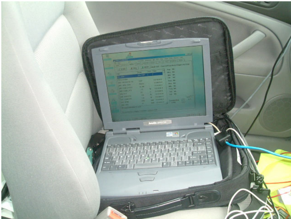
Figure 4: Laptop and OBD output
