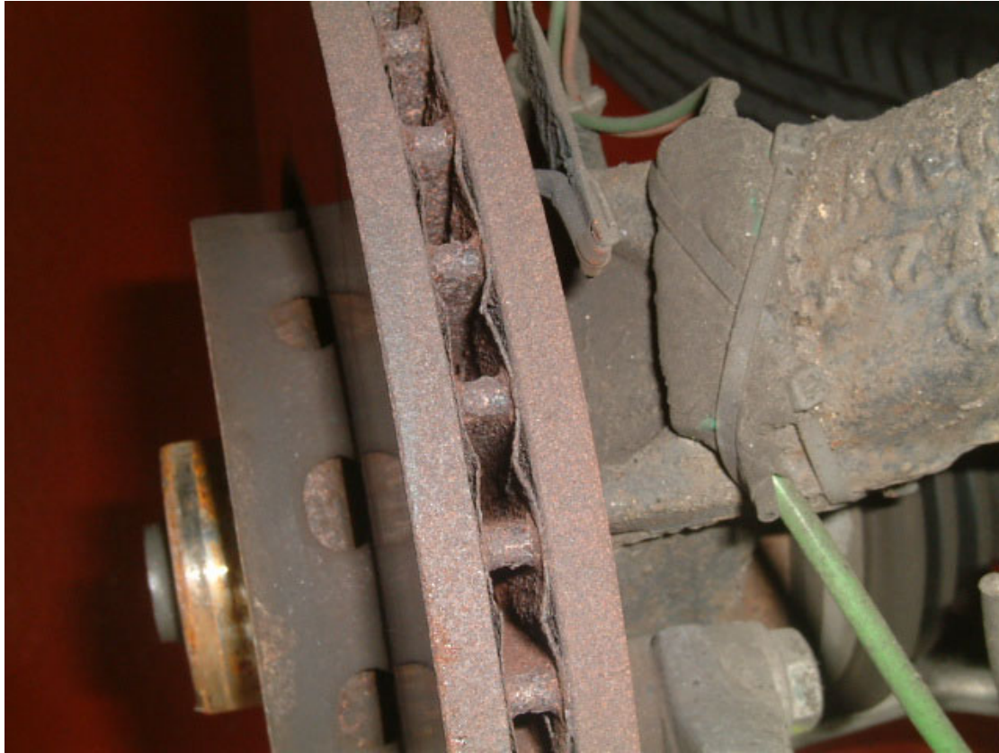
Figure 5 Contact thermocouple (touching on right side of disc, see upper middle area of figure)
