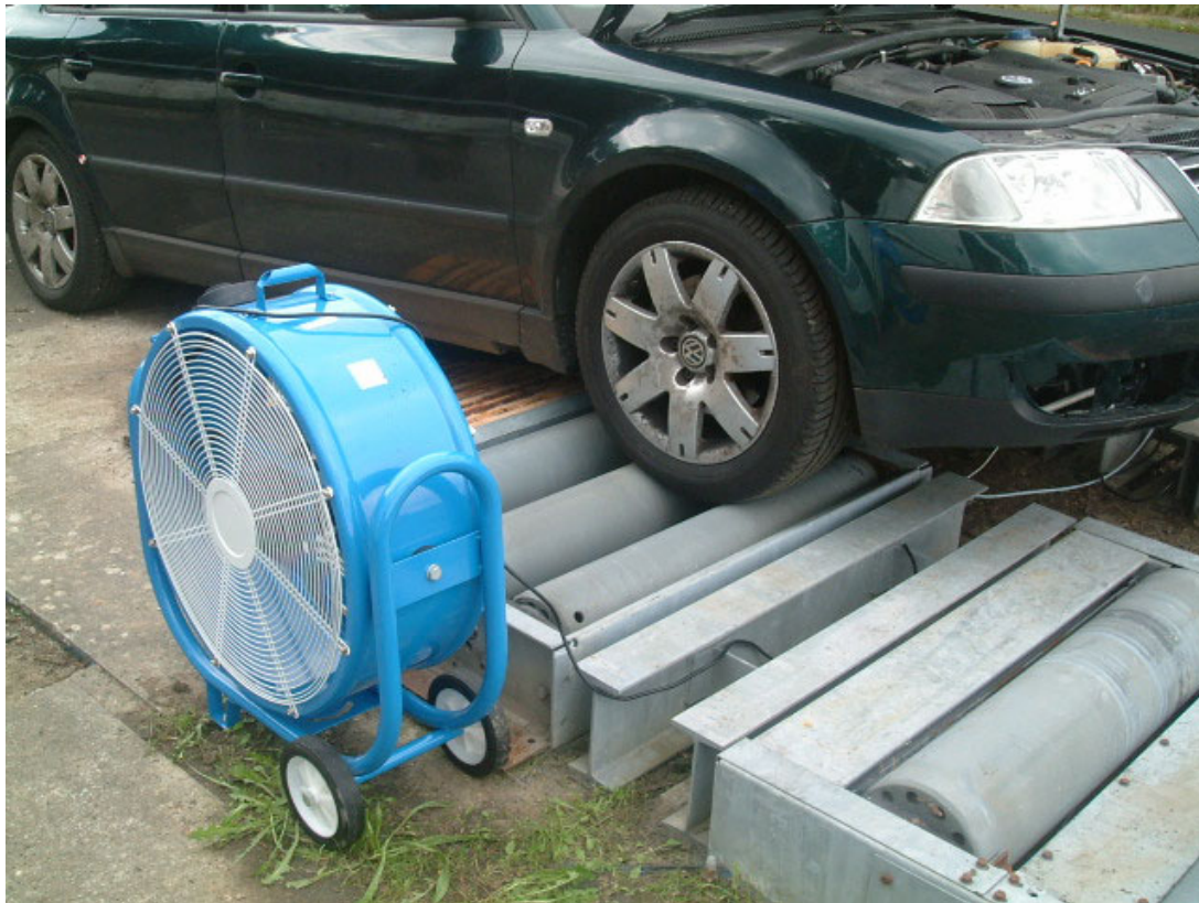
Figure 1: Roller assembly and cooling fan
