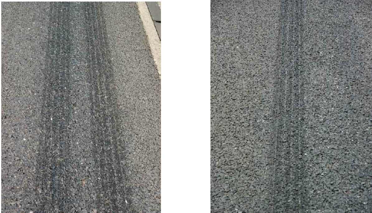
Figure 2.7. Normal tyre, normal pressure (left – showing the marks from two successive runs) and +30% pressure (right):
