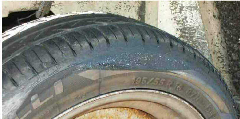
Figure 2.14. Run flat tyre with wear to shoulder after fully deflated runs
