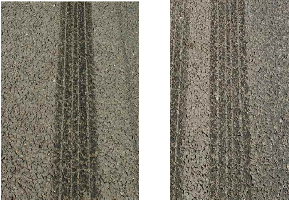
Figure 2.12. Run flat tyre, +30% pressure (left) and -30% pressure (right)
