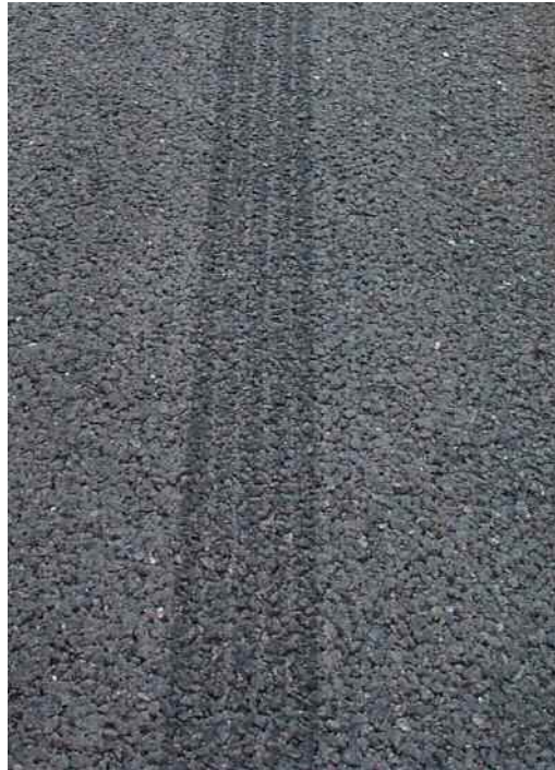
Figure 2.8. Normal tyre, -30% pressure
