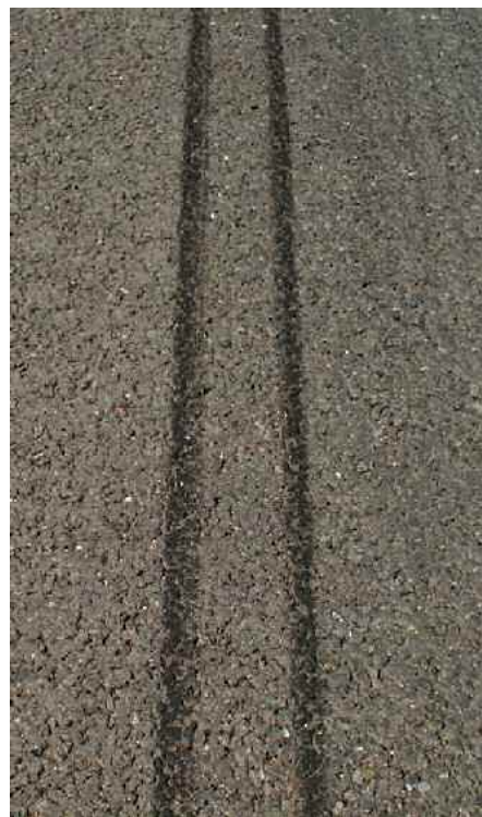
Figure 2.13. Run flat tyre, fully deflated
