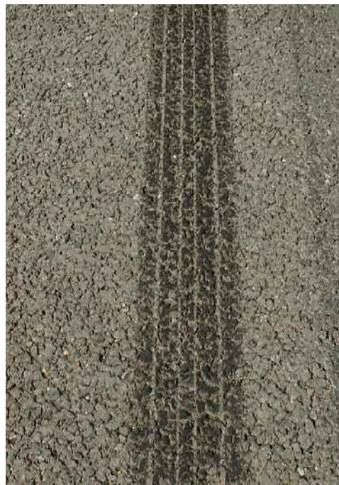
Figure 2.11. Run flat tyre, normal pressure
