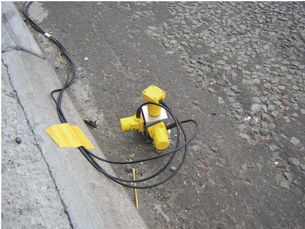
Figure 2.3: Geophone array mounted on the road surface with Plaster of Paris
