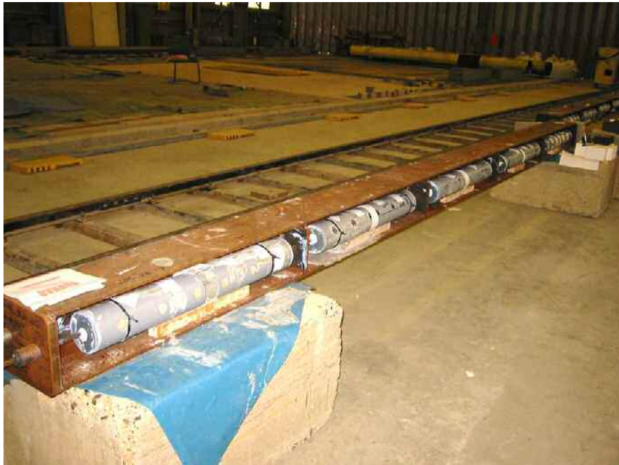
Figure 1 Layout and type of void on stressed tendons
