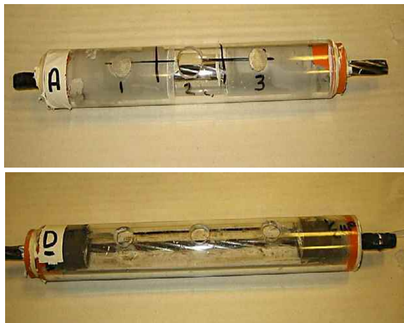
Figure 5 Examples of unstressed specimens: centre void (upper), grout halfway up the tendon (lower)
