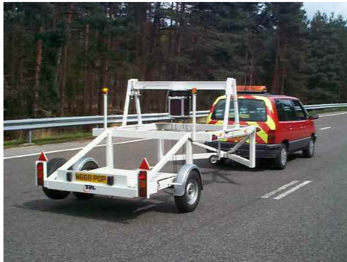
Figure 4: Trailer arrangement and towing vehicle used for performing static and dynamic measurements of absorption coefficient
