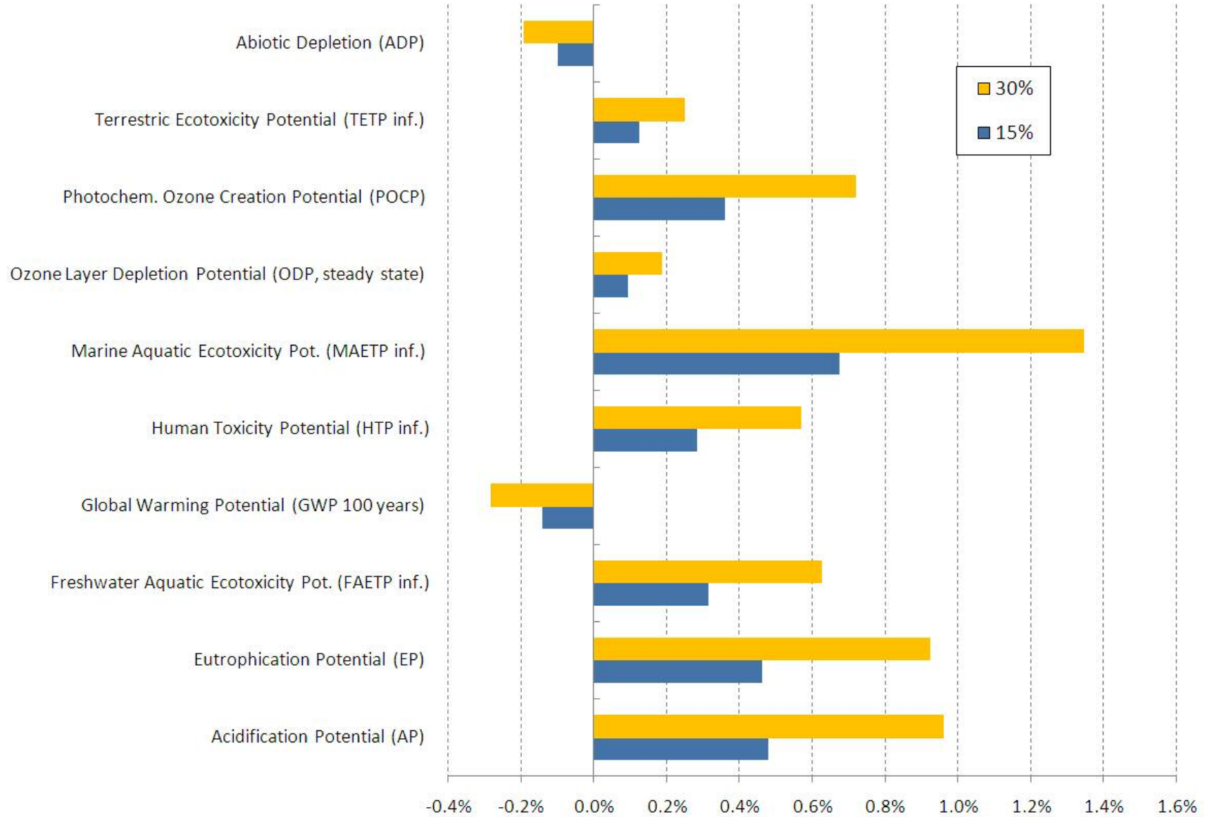
Figure 6. Impact profile for a highway containing 15% and 30% glass in the binder layer
