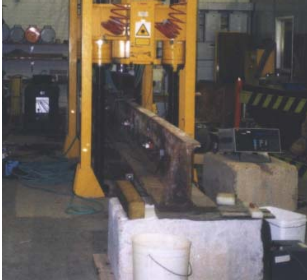
Figure 4 Cast iron beam under test rig
