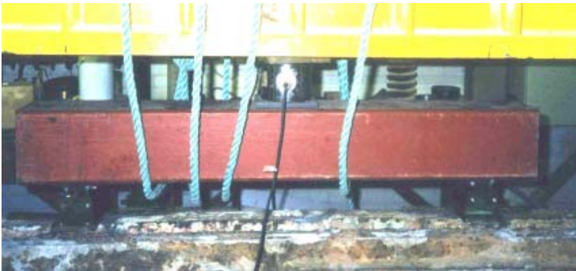
Figure 5 View of load cell and spreader beam
