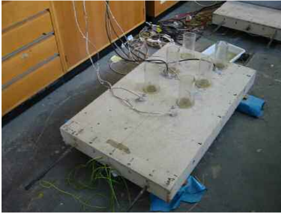
Figure 3 Ponding tubes on Specimen B
