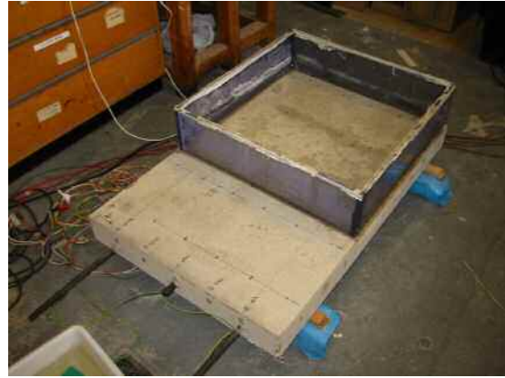
Figure 4 Ponding reservoir on Specimen A
