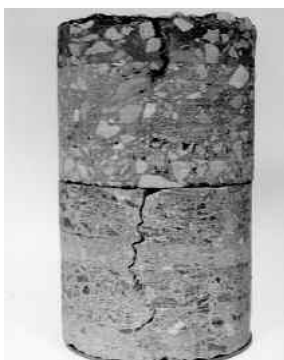
Fig. 1 Core from recently initiated reflection crack
