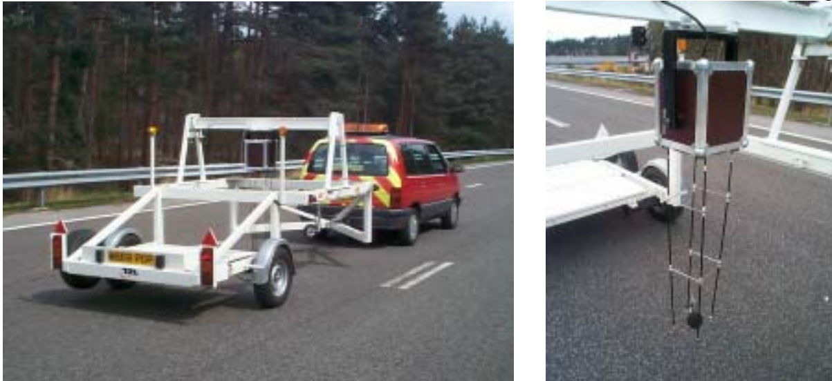
Figure 2: The MLS trailer system and the loudspeaker/microphone arrangement
