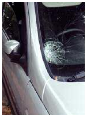
Figure 3-17. Evidence of impact to windscreen and dent in A-pillar
