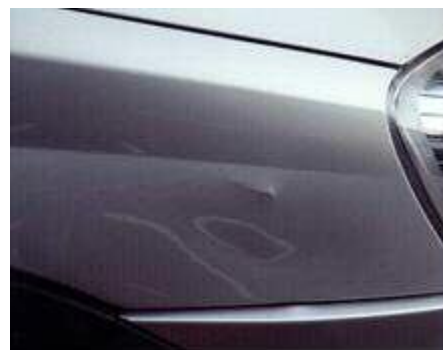
Figure 3-18. Damage to front offside wing
