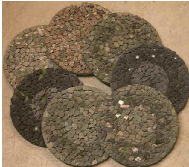
Figure 1 Aggregate specimens after polishing
