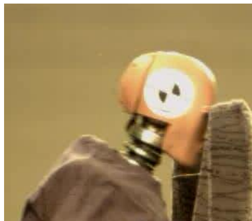
Figure 3.1.1: Moment of impact between passenger face and the seat in front impact as may be experienced in a bus or train seat impact.
