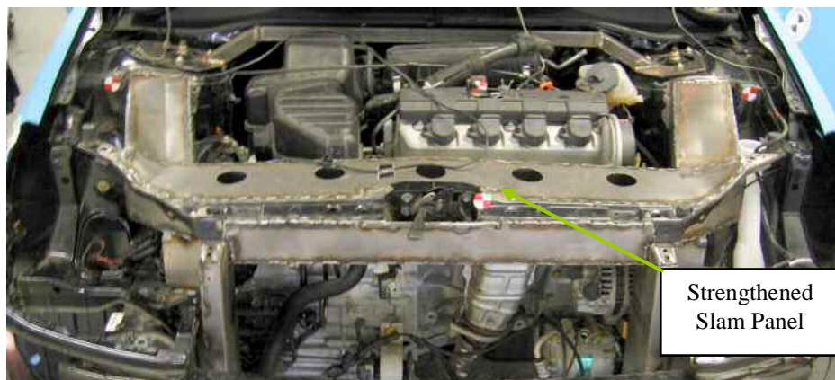
Figure 18: Revised centre section of the slam panel crossbeam connecting the leading edges of the additional upper rails across the vehicle front.
