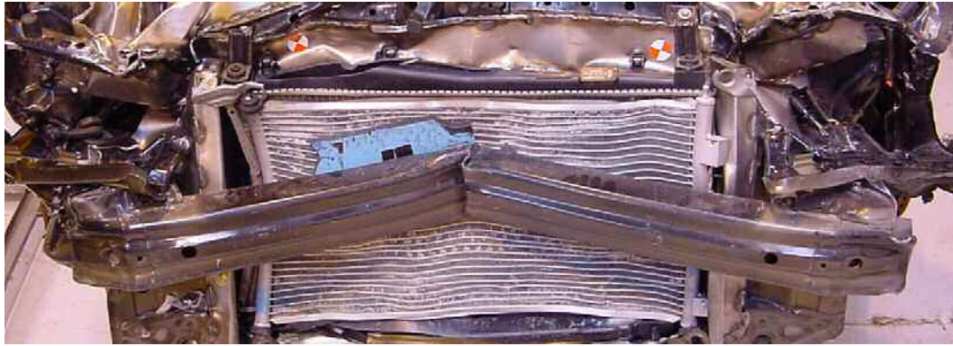
Figure 34: Bumper crossbeam deformation showing the single plastic hinge failure at the vehicle centreline.
