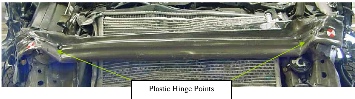
Figure 12: Bumper beam post impact showing the location of the hinge points allowing rearward translation relative to the lower rail leading edge due to loading by the barrier face.
