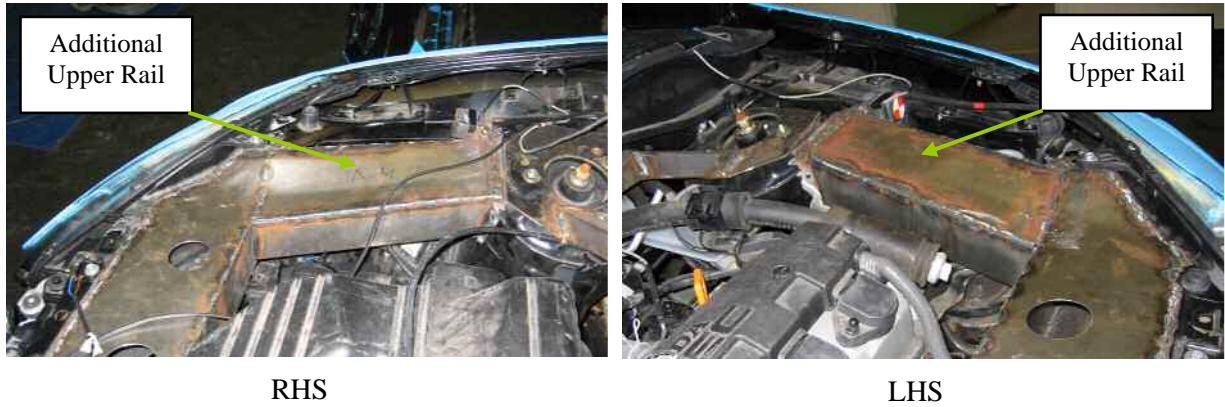
Figure 17: Additional upper rail load paths connecting at the leading edge to the centre section of the revised slam panel and at the rear edge to the front face of the suspension turrets.
