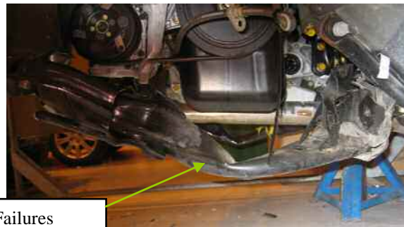
Figure 32: Lower rail load path deformation showing failure in bending about the vertical axis at different locations for the RHS and LHS. The level of deformation is visually less than for the unmodified test car.
