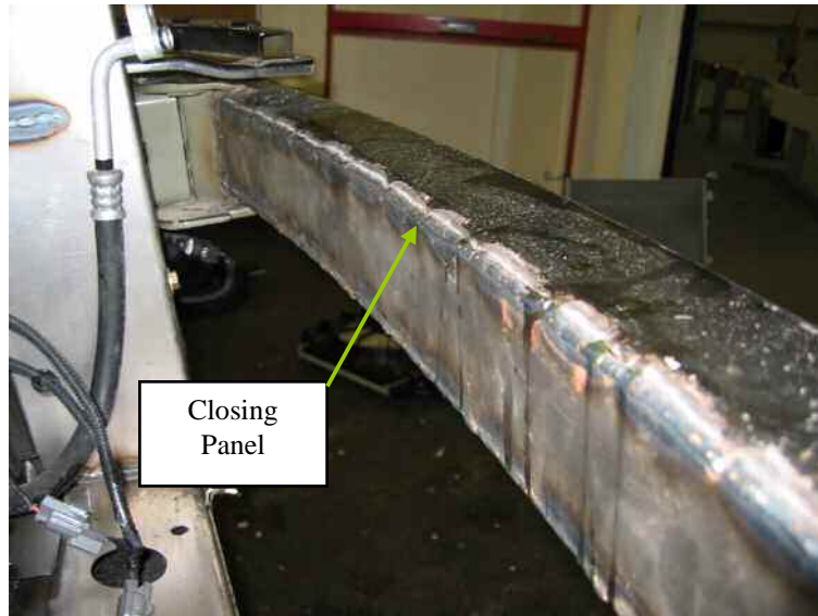
Figure 19: Front crossbeam closing panel welded onto the existing bumper crossbeam.
