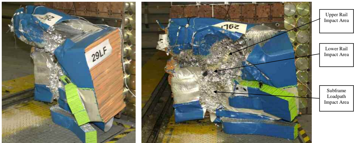
Figure 16: Resultant deformable barrier face deformation showing the approximate impact locations of the main structural load paths.
