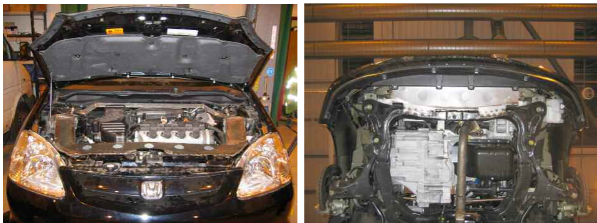
Figure 22: Front and underside view of the modified test car showing integration of the additional structure.
